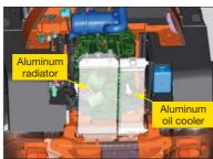
The aluminum radiator and oil cooler are located side by side for easy cleaning.
