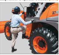
There are handrails and large steps mounted on both the left and right of the operator's station for easy access.
