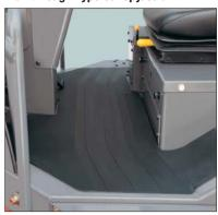
The walkthrough type canopy/cab allows for easy access from either side. The flat floor enables easy cleaning.
