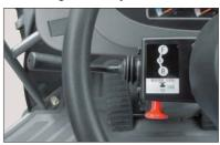
If the forward/reverse is not in neutral (N), the engine cannot start, enhancing safe operation.
