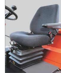
A long-stroke suspension seat, which well absorbs shocks and vibration, is optionally available.
