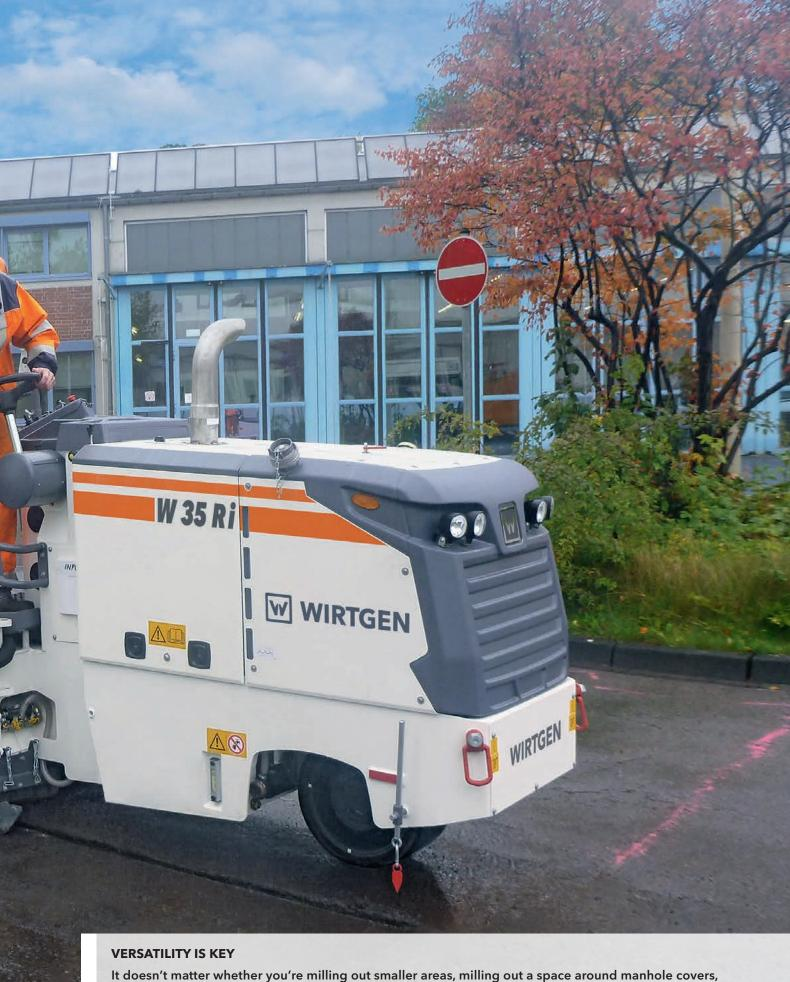
It doesn't matter whether you're milling out smaller areas, milling out a space around manhole covers, marking road surfaces and removing markings, or doing fine milling work in combination with a large milling machine. Equipped with different milling drums and WIRTGEN's innovative cutting technology, the versatile W 35 Ri small milling machine has the right answer to nearly every challenge.
