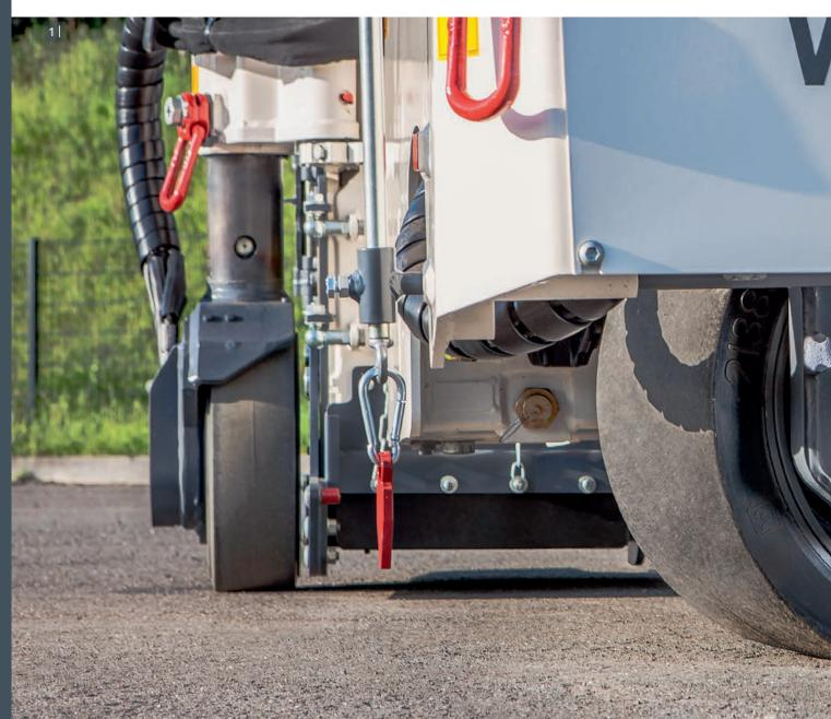
2 The small milling machine is ideally suited for fast maneuvering in narrow areas - also thanks to the ability to simply swing in the right rear wheel.
