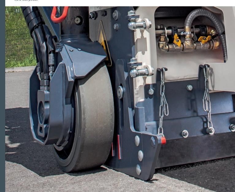
2 The sprinkler unit is easily accessible and the individual spray nozzles can be easily removed for cleaning.
