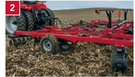
Disk gang depth: slice, cut and bury residue to the producer's desire.
