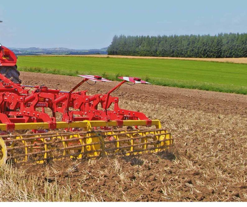
SYNKRO K models are equipped with hydraulic folding and mechanical transport interlocks.
