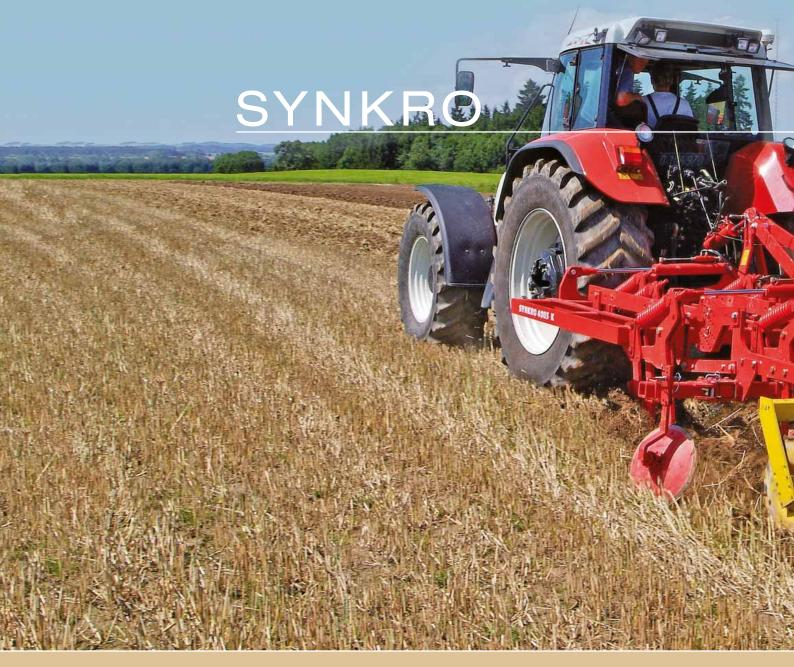
These three-row cultivators have been designed so they can be used for both shallow and deep soil cultivation (up to 11.8" / 300 mm.
