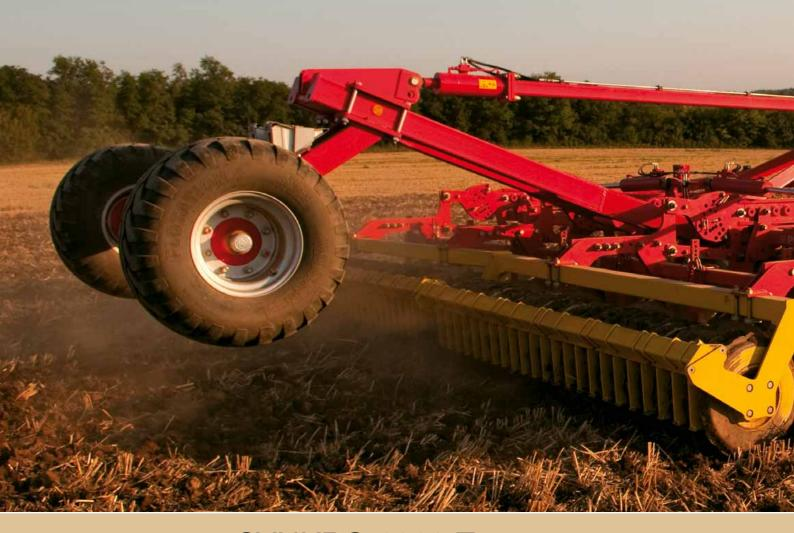
A transport chassis carries the machine, resulting in less weight on the linkage protecting the tractor.
