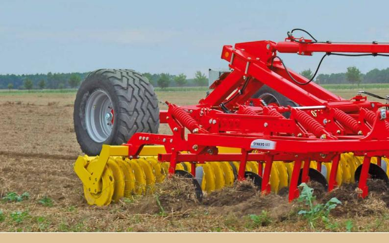
The length and angle of the drawbar are adjustable. An ideal match to every tractor and rear roller is ensured as a result. This optimised mounting geometry improves ground clearance at headlands and during transport.
