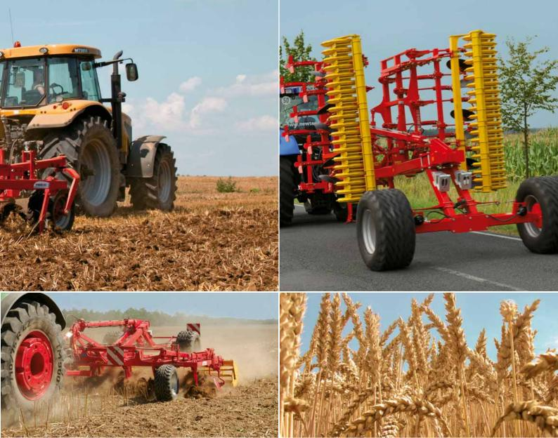
The SYNKRO series cultivators are designed so that they can be used for both shallow and deep soil preparation (up to 12" / 300 mm).
