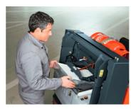
Clean exhaust air and long operating times: Cassette filter system with a large filter surface and Hako's patented R<sup>2</sup>S filter-cleaning technology.
