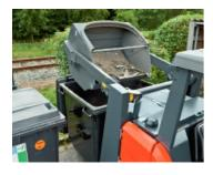
Hydraulic dirt hopper lifting system: The dirt hopper can filled to 100% and allows high dumping at heights of up to 142 cm.
