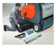
Convenient sweeping cylinders: Tool-free changing of the sweeping cylinder, and protection against wrapping to prevent bearing damage when sweeping up plastic films and straps.
