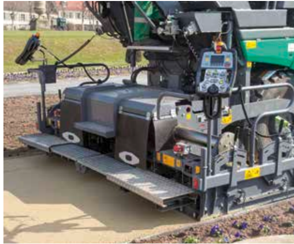
AB 340 TV with 25cm bolt-on extensions
