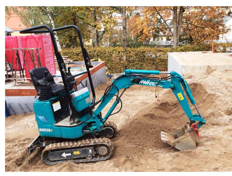
**Engine netpower:7.2kW Machine weight:1010kg**
