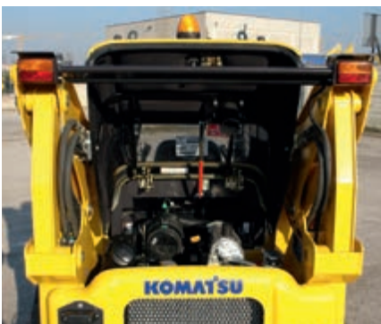
The bonnet: quick engine check
