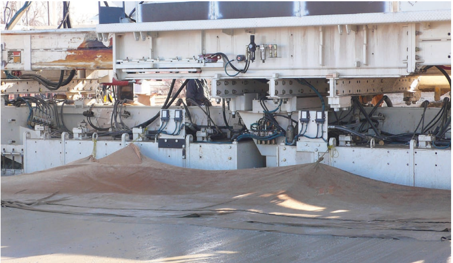
Vibrator manifolds mounted on kit minimize assembly and disassembly time: less hydraulic hoses.
