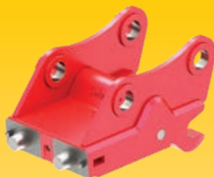
Mechanical quick-coupler MS10 Durable and reliable even in heavy-duty operations. Locked by turning a socket wrench, safely locked over dead point.
