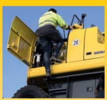
Handrails and anti-slip plates
