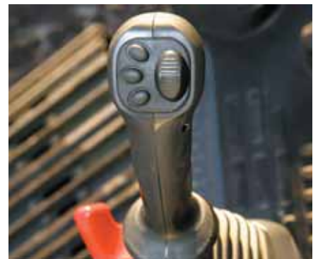
Joysticks with proportional control button for attachments
