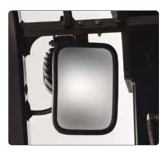
Flat or convex mirrors are available in a selection of shapes and sizes, including round, rectangular and wide-width. Yale mirror options include a universal mounting bracket to help achieve a proper fit on the round or rectangular tubing of overhead guards.
