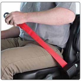
Yale also offers an interlocked option of the high visibility seat belt which disables truck travel if the seat belt is not latched. A sequencing interlocked version is also offered, which requires a step-by-step start-up procedure to prevent the seat belt from being latched prior to the operator sitting in the seat (out-of-sequence operation disables truck travel).
