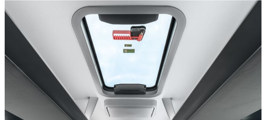
Large, translucent and tinted glass skylights
