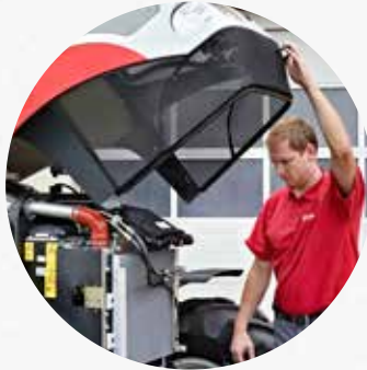
One-section bonnet on gas struts can be raised, even when a front-mounted implement is attached.
