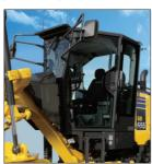
ROPS (Roll-Over Protective Structure) Cab (Equipped with defroster and intermittent wiper)
