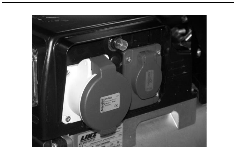
Fig. 3-2: Connecting up consumers/appliances
