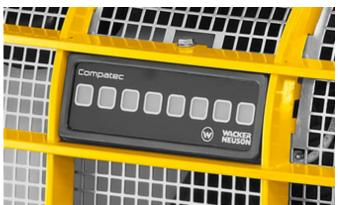
Optionally available with shutdown at overcompaction or Compatec - a display which indicates the degree of compaction.
