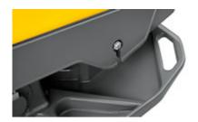
• Tie-down options similar to those of large equipment allow an optimal securing during transport
