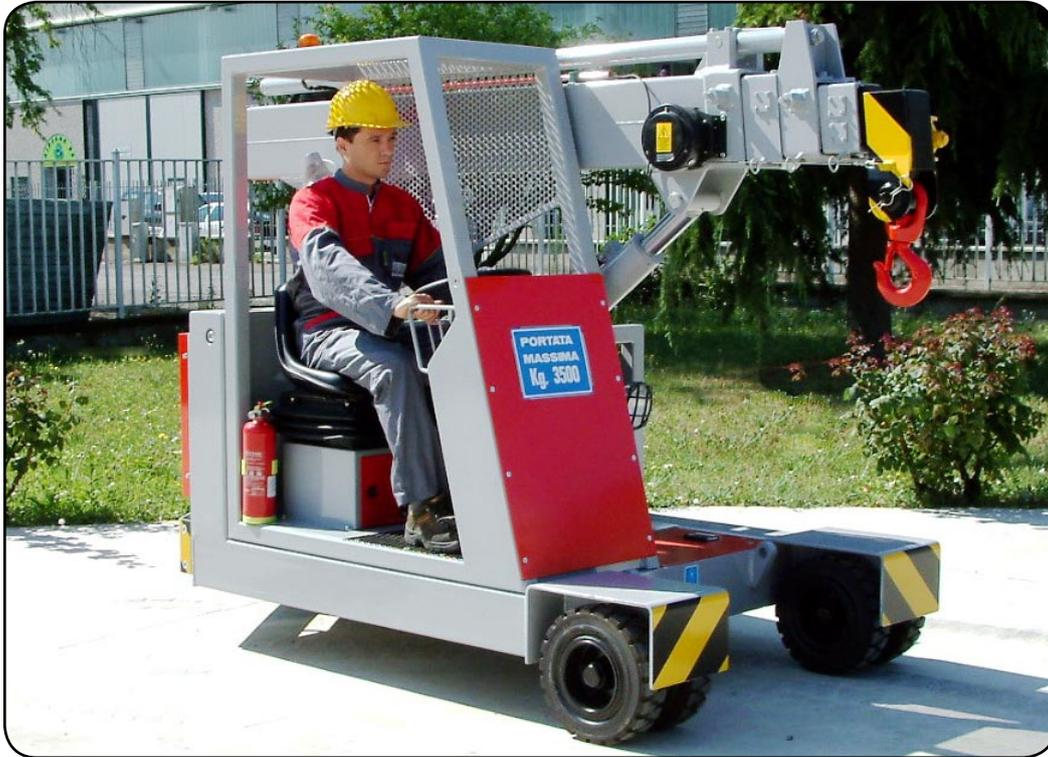
**DRIVE:** DC 3.3 kW - 24 V fanned reversible electric motor with MOSFET electronic control HF and energy saving, self diagnostic, speed and temperature checks (no. 2 thermostats), brush wear warning. Foot hydraulically operated brake to drive wheel. Hand brake mechanically operated. Gear box between motor and drive wheel in oil bath. Speed up to 8 km/h.
