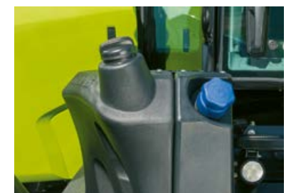
455 l fuel tank with integral 42 l urea tank.
