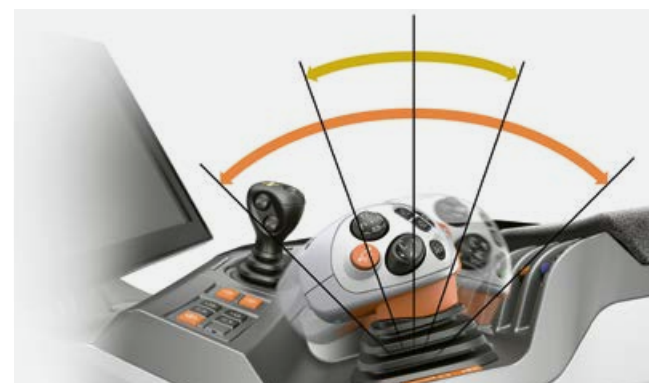
Shifting operation Powershift speeds + / - Shifting operation Range + / -
