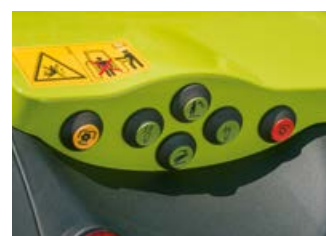
External controls for rear PTO on both mudguards
