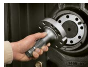
The PTO stub can be changed easily
