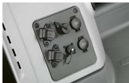
Connections to the power supply and ISOBUS for additional terminals are located below the right-hand console
