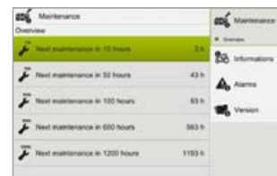
Maintenance counter in the CEBIS and CIS display
