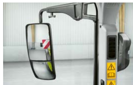
As well as the large standard mirror, a wide-angle mirror for improved road safety is supplied as standard
