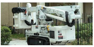
Recommended safety equipment, available through Altec Supply, include a platform liner, fall protection system, wheel chocks and outrigger pads.
