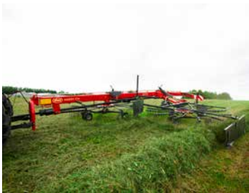
The side delivery concept allows you to collect crop from 15.00m into a single swath.
