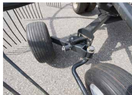
Optional tandem axle for additional stability specially on hillside.
