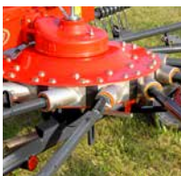
Tine arms can be easily removed.
