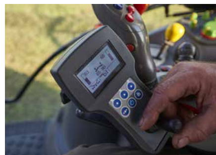
ComfortKit including electronic control of separate rotor height.
