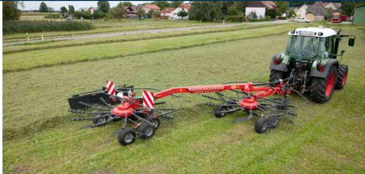
The 714T Vario with 7.10m working width and unique SideShift device.
