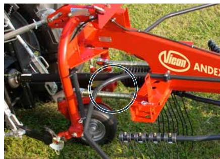
Oscillation dampers ensure excellent running characteristics.
