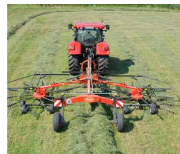
The Andex multirotor rakes are fitted with TerraLink Quattro for excellent raking. Except for Andex 644.
