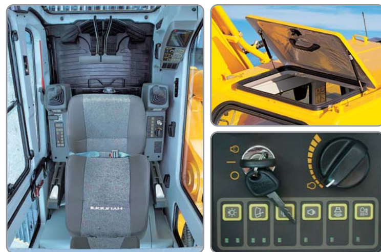
1 2 3 1 Wide, Comfortable Operating Space 2 Steel Cover Sunroof 3 Dial Type Engine Speed Switch and Key Switch
