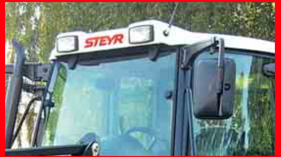
Low profile cab for extra-low clearances.
