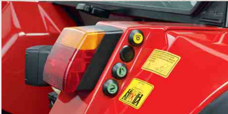
Fender controls for operating hitch and PTO from alongside implement.
