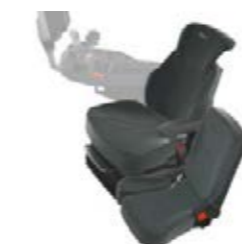
■ The comfort seat features air suspension and easy armrest adjustment.
