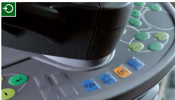
Membrane keypad for implement lock and damping activation.
