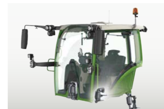
□ The pneumatic cab suspension with braking and pitch compensation reduces vibrations to a minimum and provides high ride comfort. It is supported on three points and has an integrated self-leveling feature. (available for Fendt 700 Vario Profi and ProfiPlus).
