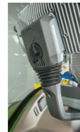
The Varioterminal can be adjusted in all directions thanks to a new bracket with a ball joint.
