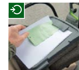
□ The instructor seat can be folded down into a table with a clamp for documents.
