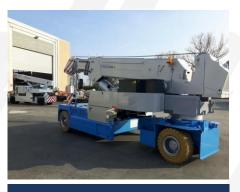
Extendable chassis to increase lifting capacity
