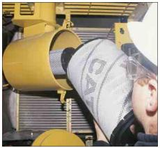
**Pump Compartment.** A service door on the right side of the upper structure allows ground-level access to the pump and pilot filter.
