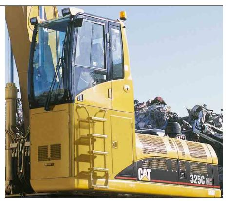
Raised Cab. The 1200 mm or 1600 mm raised cab further improves operator's visibility in all material handling applications. To reduce vibrations and sound the cab shell is attached to the frame with viscous mounts.
