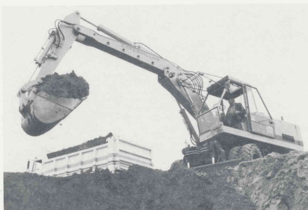
The 214 is powered by the 102 hp Perkins 6.354.4 P engine.
